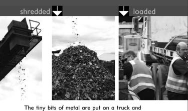
The tiny bits of metal are put on a truck and taken to a steel mill.
