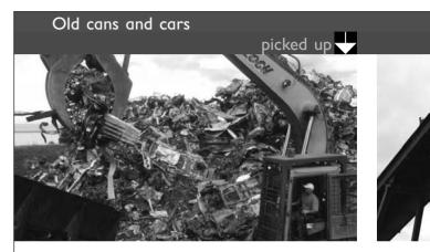
The crushed cans and cars are then picked up by a machine and put through a shredder. The shredder cuts them into tiny bits of metal.
